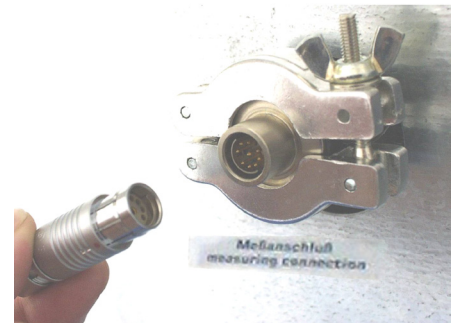
Figure 28: Measuring connection (15) with measuring access port and supplied plug
