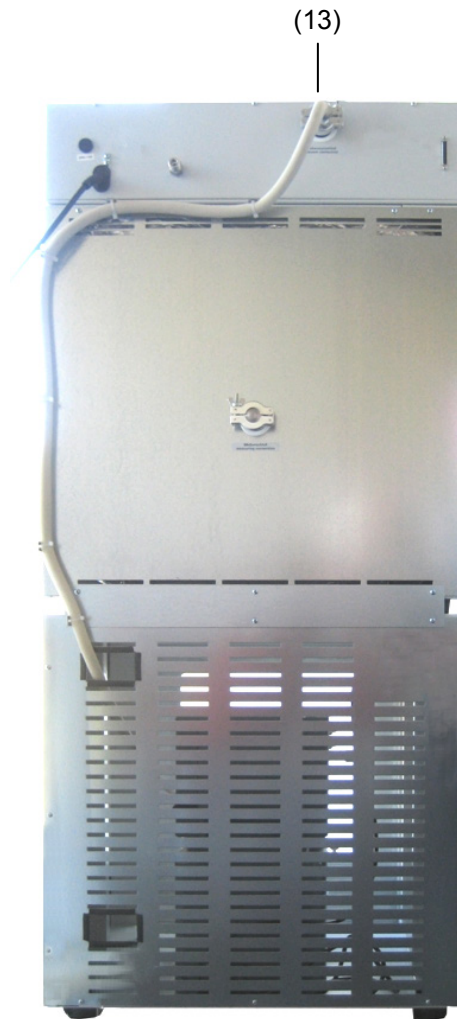
Figure 20: VDL 53 with option vacuum module with pump
