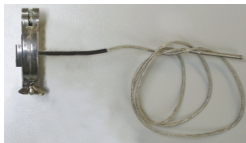
Figure 26: Measuring current port with universal eccentric ring and locking ring DN 16, with flexible Pt 100 temperature sensor
