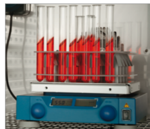
Shaker operation in the chamber
